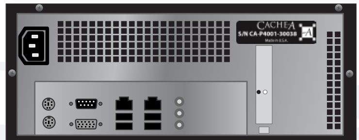
Power Service Mouse Service Keyboard Monitor Gb E 1 USB3 USB4 Gb E 0 USB5 USB6 Tape SAS Adaptor
