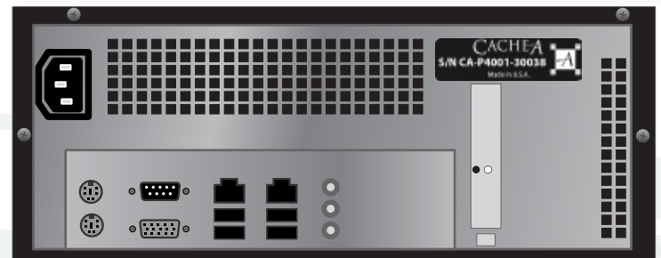
Power Service Gb E 1 Gb E 0 Tape Mouse Service USB3 USB5 SAS Keyboard Monitor USB4 USB6 Adaptor
